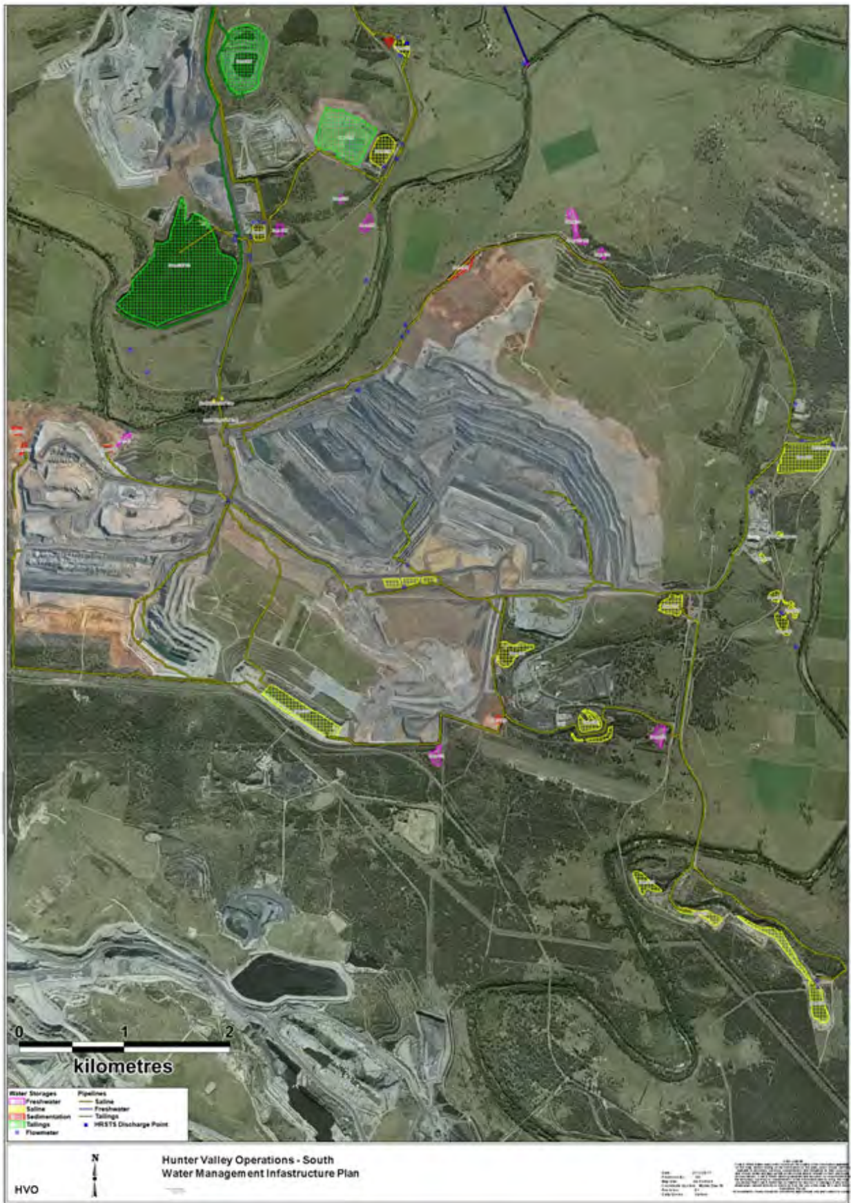
Figure 22: South Pit water management infrastructure
